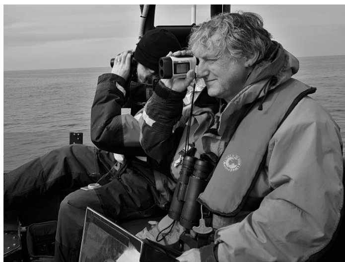
Figure 1. Use of Nikon Forestry Pro laser rangefinder during a boat-based survey.
