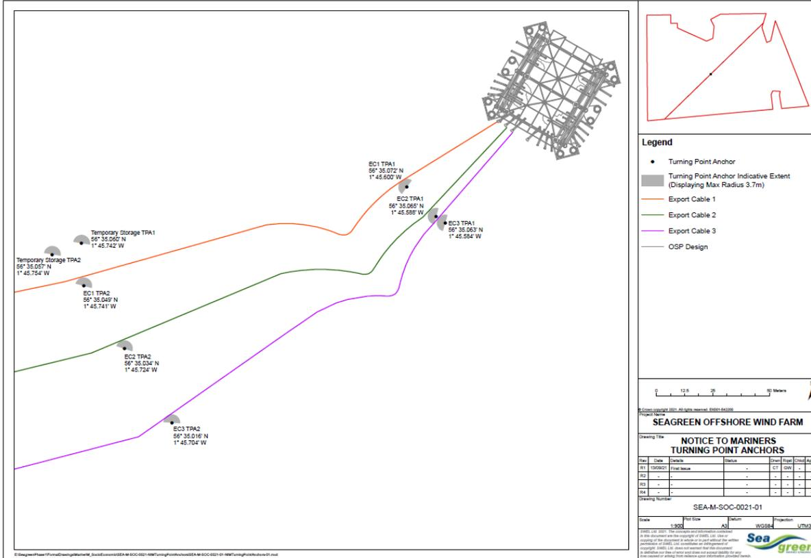
Fig 6 – Turn point anchor wet-stow and deployment positions
